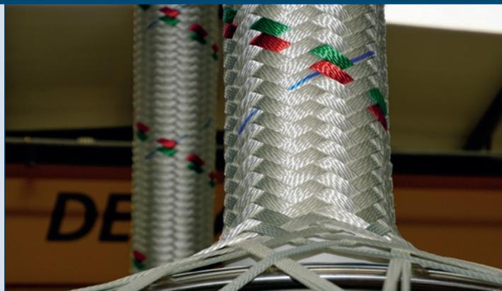
Lankhorst Offshore manufactures deepwater mooring lines based on Cabral® 512 polyester ropes. They utilise high efficiency sub-rope cores laid parallel within a filter system and an outer braided jacket. Each sub-rope is monitored during rope manufacture to ensure all sub-ropes have equal tension and length. Typically, Cabral® ropes include 7 to 18 sub-ropes dependent on the mooring project; each sub-rope is a braided construction, giving a 100% torque free rope.
