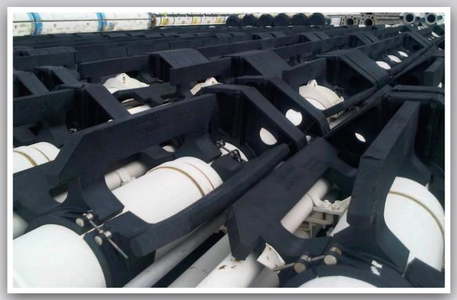
Protection and storage of bare drilling risers strings both on and offshore can often be an issue, Lankhorst Mouldings provides solutions for both.
