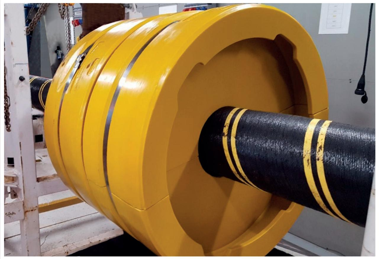
Lankhorst's Clearance Protection system consists of cylindrical half shells moulded from high impact resistant polyurethane (PU) or polyethylene (PE) material, and is available in a wide range of inside diameters, lengths and clearances. The system is designed to provide clearance between two cables or pipelines when they cross each other, as an alternative to concrete mattresses or rock dumping.
